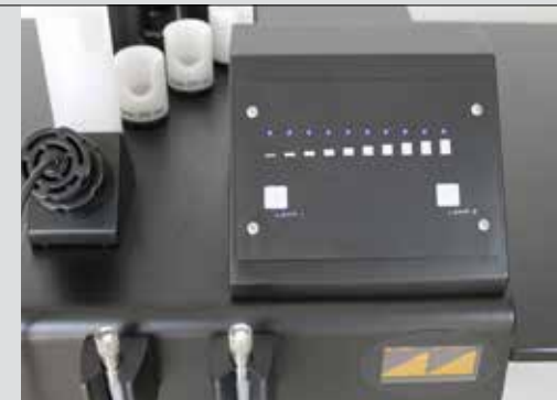
Integrated led light source with double outlet and n.2 fiber optic cable. Colour temperature of 5.500°K/200 lumen. Brightness intensity regulation by Soft Touch Control Panel.
