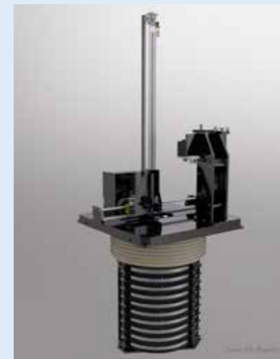
Detail of a disc to store cryotubes inside LN 2 tank
