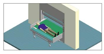
**2.** The patient is collected from the stretcher by the contemporaneous movements of belt rotation and transfer top translation. The table top is lifted up to the maximum height to allow the removal of the stretcher and at the same time the opening of the window (if present).
