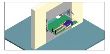
**3.** Table top transfer from the septic to the aseptic area. Collecting, lifting up and transferring the patient and closing the window can be done manually or sequentially. Such operations can be managed by only one operator.
