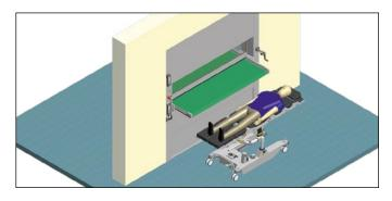
**6.** Table top is lifted up to the maximum height to allow the removal of the operating table with the patient on it and at the same time the window closure (if present). The operations of downloading, lifting up, and closing the window can be done manually or sequentially.
