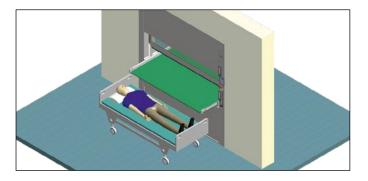
**1.** The stretcher with the patient is moved closer to the patient transfer unit Gamma/1, adjusting the height of the platform. The correct positioning is done by pressing the button" transfer top down" and, depending on the PTU model, by the sensors that detect the stretcher.
