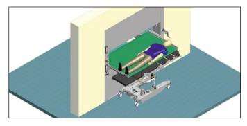
**4.** The operating table is moved closer to the PTU, checking the height of the transfer top and the patient's position. The correct positioning is done by means of the button "transfer top down" and, depending on the PTU model, by the sensors that detect the operating table.
